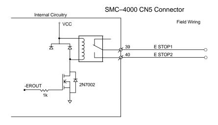
The SMC–4000 closes the relay contact under normal operating conditions. The relay is controlled by the same circuit as the error LED. The relay will be open if the error LED is ON.
