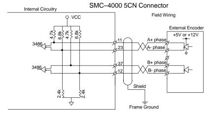
X axis internal encoder shown See 5CN connector for other axis pin connections.
