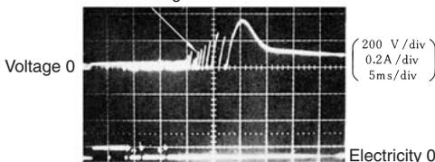
(b) DC Breaking Characteristics of Conventional Power Relays
