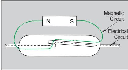
● Magnetic and Electrical Circuits of Bestact
